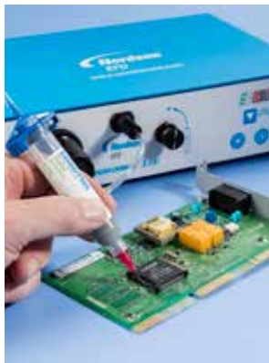
Dispensing SolderPlus® solder paste on PCB boards.
